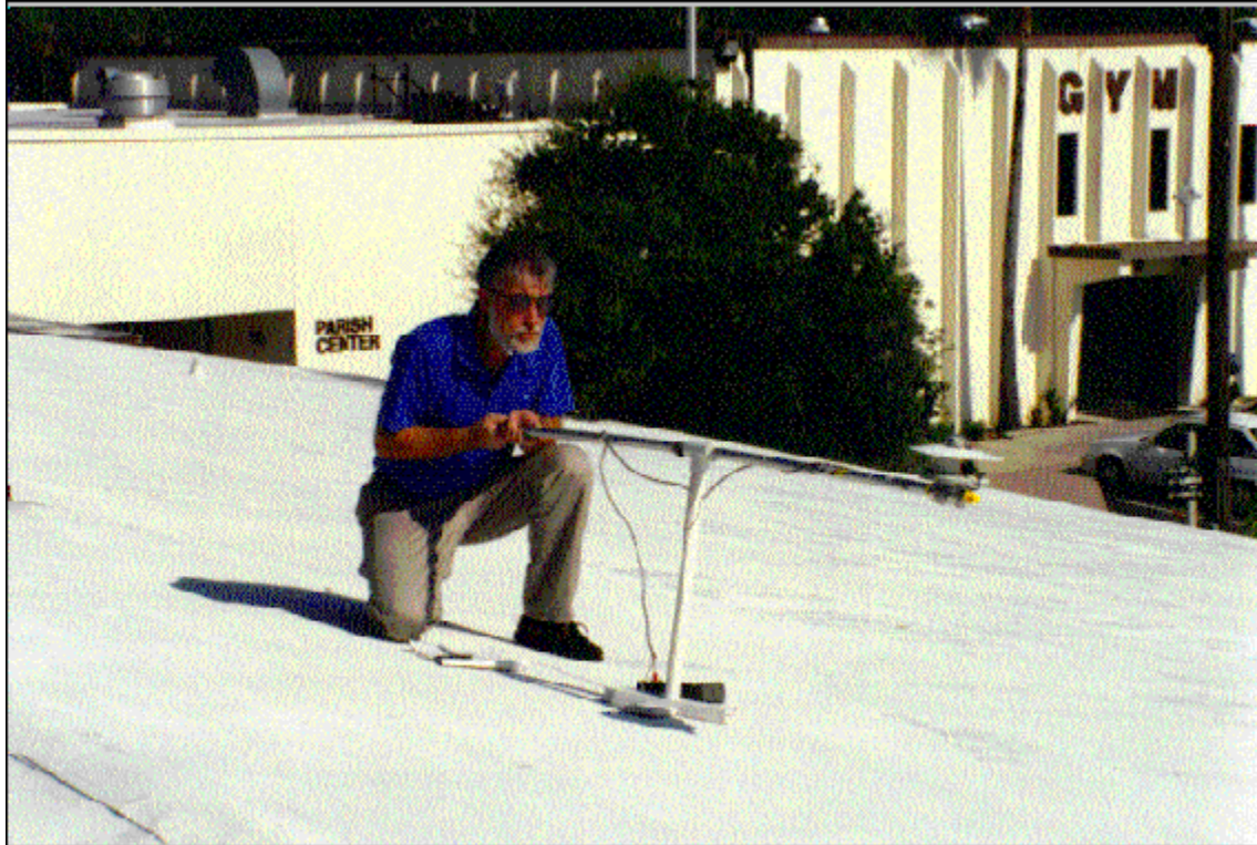
Figure 11. Pyranometer is used to measure roof reflectance one year after initial treatment.
